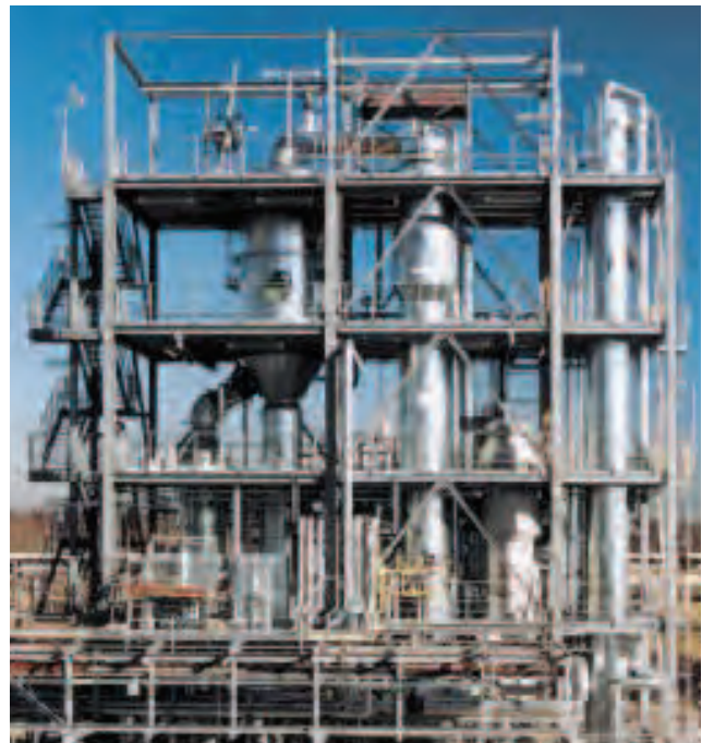
2-effect falling film, forced circulation evaporation plant in counterflow arrangement with downstream system for the purification of vapour condensate by distillation of waste water containing salts and organic compounds. Evaporation rate: 9,000 kg/hr concentrated to 65 % TS
